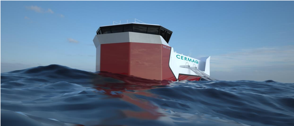
VARD 8 54 Offshore fish farming operation platform | Overall length: 36 m | Breadth: 12 m | Designed by Vard Design
