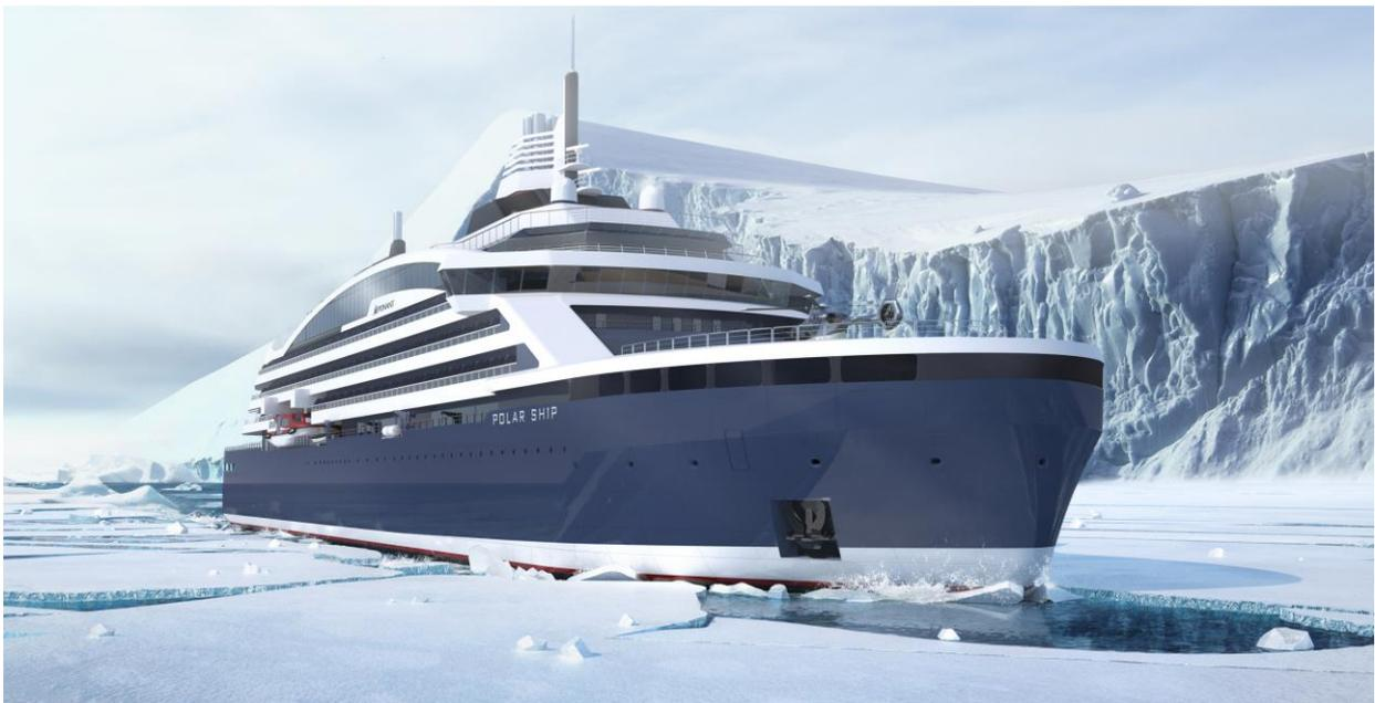
**VARD 6 17** Electric hybrid cruise icebreaker with LNG propulsion
