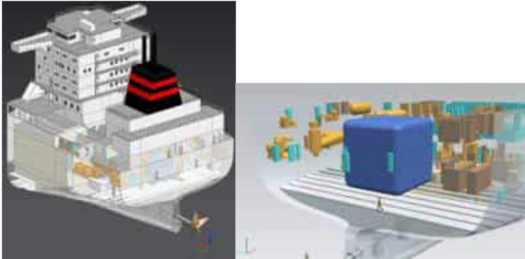
Figure 3 – Nuclear reactor (blue box) in the Cadiz Knutsen LNG tanker of Figure 1.
